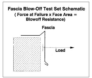
Figure 4: Fascia Test Schematic
