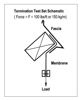
**Figure 3: Termination Test Schematic**
