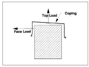
Figure 5: Coping Bi-Directional Test Schematic: Top and Face Leg.
