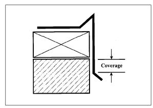
Figure 1: Edge Flashing Coverage
