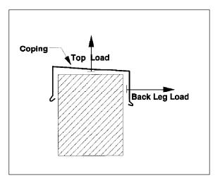
Figure 6: Coping Bi-Directional Test Schematic: Top and Back Leg.
