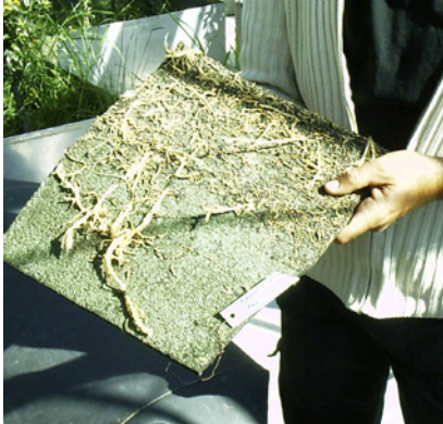
Figure 3: Root penetration on backside of Membrane
