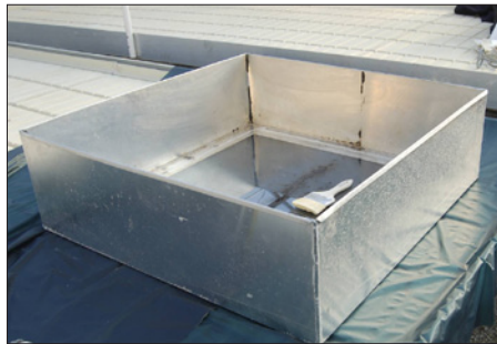
Figure 4: Sample trial container . Note the interior metal fold to support the clear Plexiglas base.
