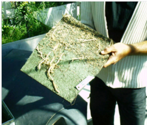
Figure 6: Root penetration on backside of tested root barrier.
