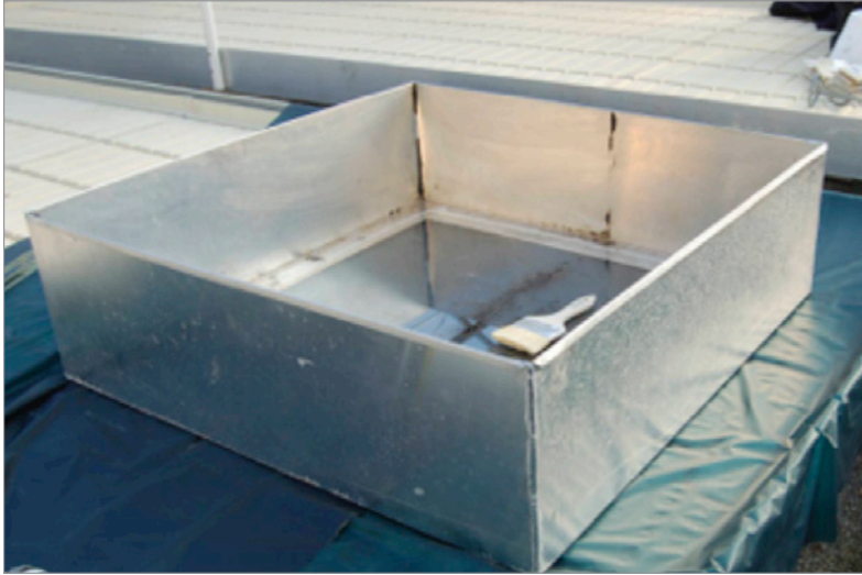
Figure 3: Sample trial container. Note the interior metal fold to support the clear Plexiglas base.
