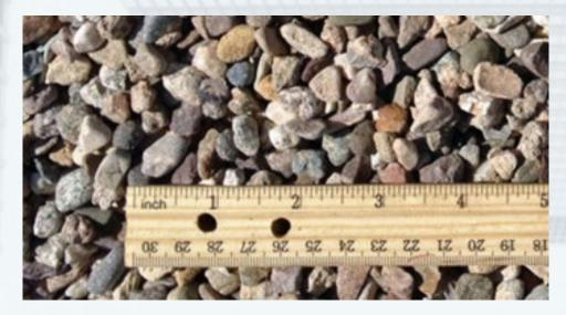
Aggregate is used with BUR material to protect the material Nom. 1/2-inch diameter
