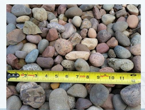
Ballast on membrane is used to hold the roof assembly down. Nom. 1.5-inch diameter
