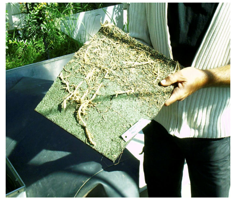
Figure 6: Root penetration on backside of tested root barrier .
