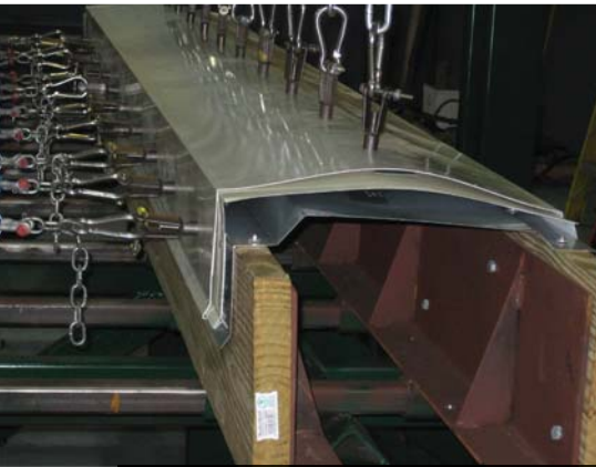
As part of the ES-1 testing protocol, RE-3 tests upward and outward simultaneous pull of a horizontal and vertical flanges of a parapet coping cap.
