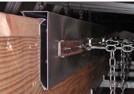
This gutter is being tested using the test method specified in ANSI/SPRI GD-1, "Design Standard for Gutter Systems Used with Low-Slope Roofs."
