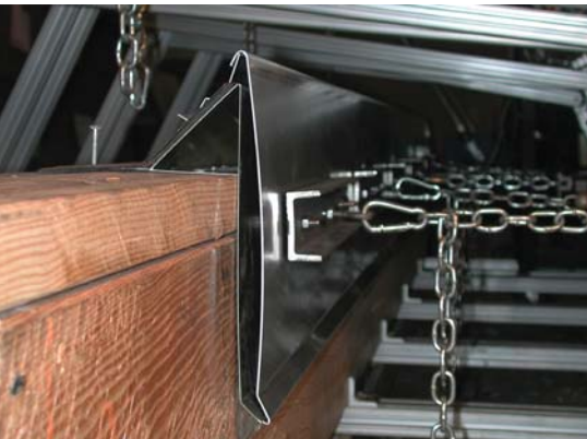
This gravel stop is being tested according to the ANSI/SPRI ES-1 standard using the RE-2 test for fascia systems.
